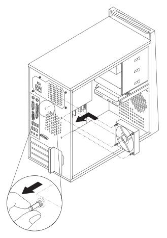
Figure 31. Installing the rear fan assembly
